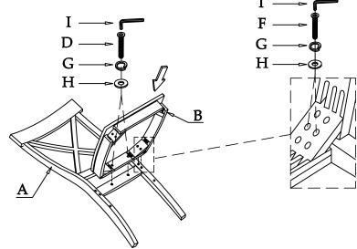
Step 2: Using the Allen Key to tighten all bolts
